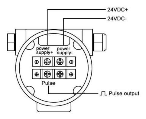
Figure 2 no display pulse output type wiring diagram
