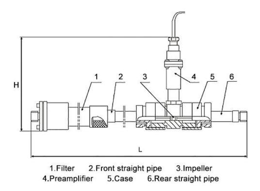
Figure 6 structure of SUP-LWGY turbine flow meter
