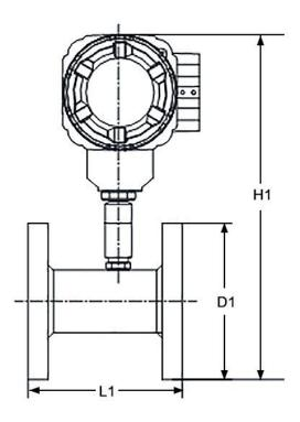
Figure 8 flange connection type
