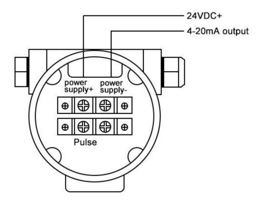
Figure 5 intelligent display 4-20mA current output wiring diagram
